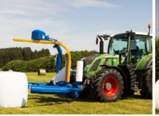
The additional equipment "Bale tipper" is used to position the bale on its front side.
